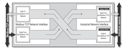
Each buffer holds a maximum of 256 bytes of data. The first two bytes in either direction can be dedicated for control/status information, and another eight bytes of data retrievable from the X-gateway by the Modbus RTU network can feature a live list. Please note that the actual number of bytes that can be exchanged is highly network dependent.
