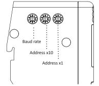
Allowed node address range is 1 - 127. Addresses 1 - 99 are available using the address rotary switches. To set e.g. node address 42, set the left address switch to 4 and the right address switch to 2. Cover the switches with the enclosed switch covers to ensure EMC compliance.
