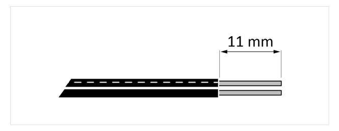
On the two wires, strip off 11 mm (7/16 inch) of the isolation.
