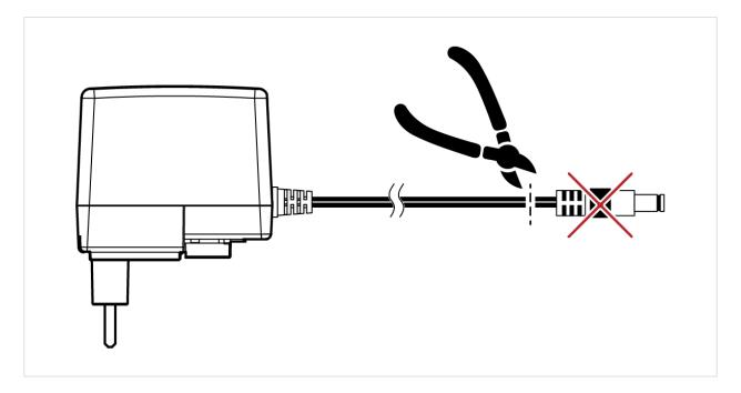
Cut the power cord to remove the existing cable connector.
