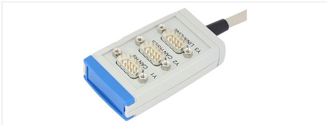
Fig. 9 Breakout box for X1 to X4
