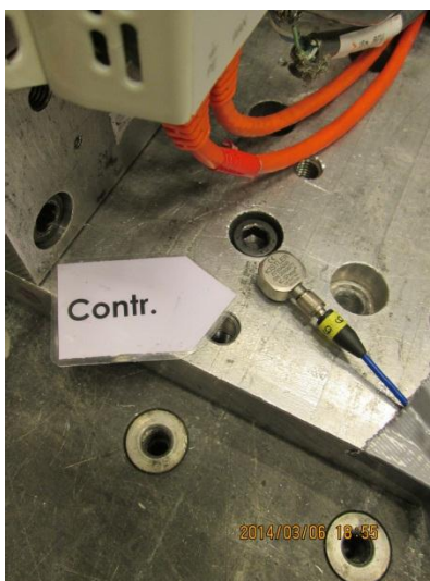
Image 18 and image 19. Control accelerometer position for Shock test A and B, X-axis and Y-axis, Z-axis
