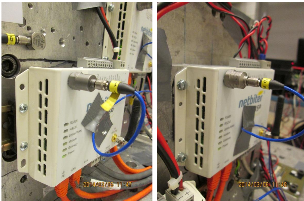
Image 8 and image 9. Measuring accelerometer positions for Sinusoidal vibration test, Y-axis
