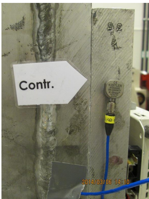
Image 11 and image 12. Control accelerometer positions for Sinusoidal vibration test, X-axis
