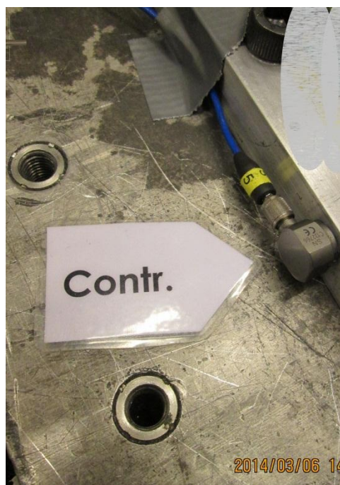
Image 11 and image 12. Control accelerometer positions for Sinusoidal vibration test, X-axis
